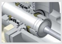
**Double Mechanical Seal in Tandem Arrangement**
